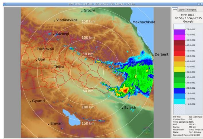
Fig. 11. Fragment of the radar picture of cloudiness above Azerbaijan 16.09.2105 in 0 hour 56 min.
