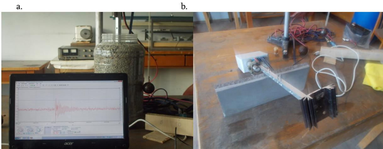
Fig.4. a) experimental equipment, b) acoustic sensor with fixed aluminum rod and radiator for increasing sensitivity
