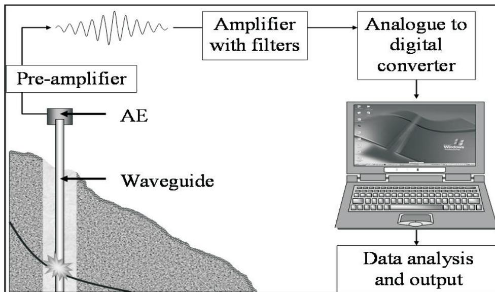
Fig. 2. Components of an AE monitoring system (Dixon et al., 2003)
