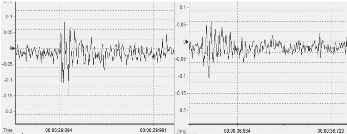
Fig.5. Recording acoustic pulses encountered in collisions on a plastic container from different distances: 1 column-sensitive sensor, 2 column-conventional sensor, a) Pendulum deviation of 25 cm, b) deviation of 20 cm, c) deviation of 15 cm, d) deviation of 10 cm; x-axis is time in sec, y-axis is the acoustic signal intensity in volts.
