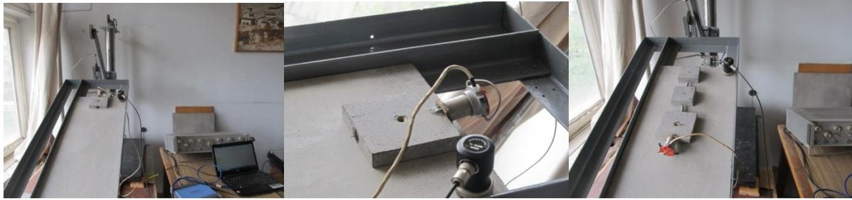
Fig. 6. Laboratory model for series of Burridge-Knopoff experiments, under the influence of gravitational forces. Middle figure shows the seismic vibrator attached to sliding plate.
