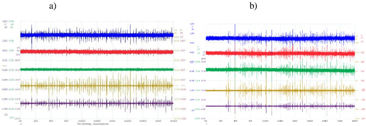
Fig.3. The Burrige-Knopoff system experiments accelerometers and acoustic emission data recordings: a)one plate and b)three plate experiments.
