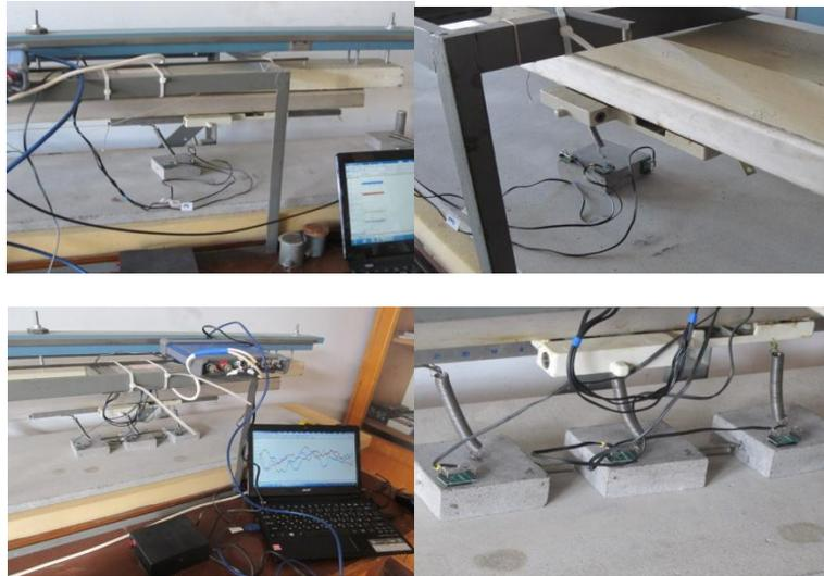
Fig.2. The Burridge-Knopoff one- and three plate experiments
