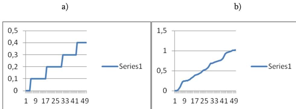
Fig. 9. a) Numerical simulation of displacement (ordinate) versus time (abscissa) for one block, b) the same calculations carried out for moving the center of gravity of the system in conditional units the Burridge-Knopoff model of four plates. (abscissa - time, ordinate - displacement).
