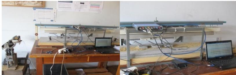
Fig.4. The Burrige-Knopoff experiments with clean surfaces plates and with a layer of sand between the plates
