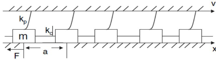
Fig.1. The schematic presentation of Burridge-Knopoff model
