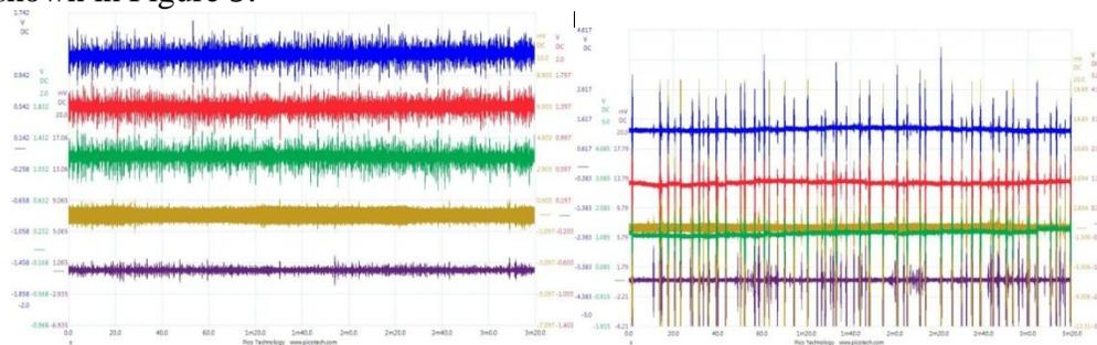
Fig. 5. Records of accelerations and acoustic emissions arising during the Burrige-Knopoff experiments with clean surfaces plates (a) and with a layer of sand between the plates (b). Blue, red and green channels, show respectively accelerometer records attached to the first, second and third sliding plate. Yellow and purple channels present the piezo sensors records.
