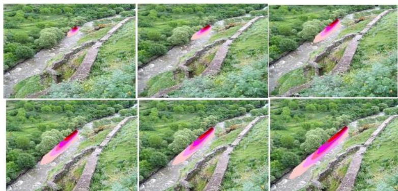
Fig. 4. The pattern of distribution of the polluting agents in section 1 within first 6 min. The step \Delta x = 20 m.
