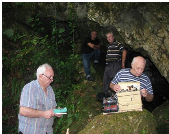
Fig. 4. Measurement of the radon and light ions concentration at the entrance into the cave. In the foreground: A. Amiranashvili (to the left) and V. Chikhladze (to the right).
