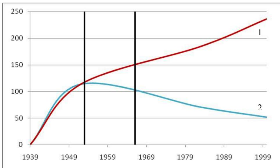
Fig.6 . Curves of sediment accumulation in Rioni River new Delta. Vertical lines indicate commissioning dates of Gumati HPP in 1953 and Vartsikhe HPP in 1967.
