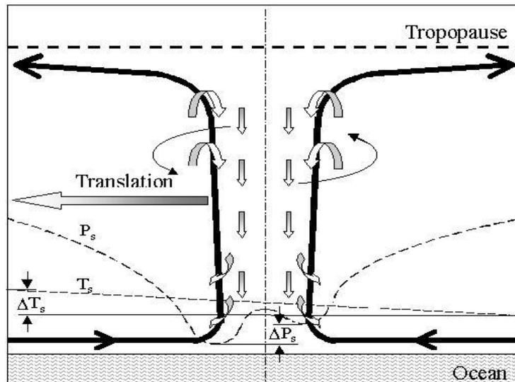
Fig. 1. The scheme of thermally powered driving mechanism.
