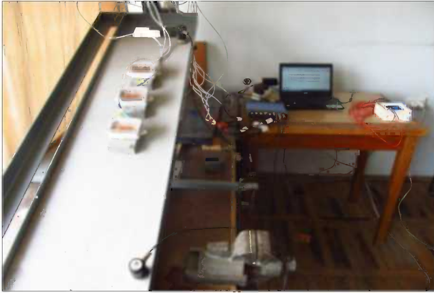
Fig. 27. The array of three accelerometers fixed on the three sliding blocks connected by springs (Burridge-Knopoff model) and placed on the lower fixed inclined block. Two AE sensors are mounted on the fixed block.
