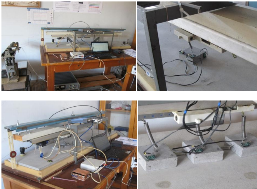
Fig.2. The Burridge-Knopoff experiments with accelerations, acoustic emissions and pulling force registration (with clean surfaces of plates and with a layer of sand between the plates)
