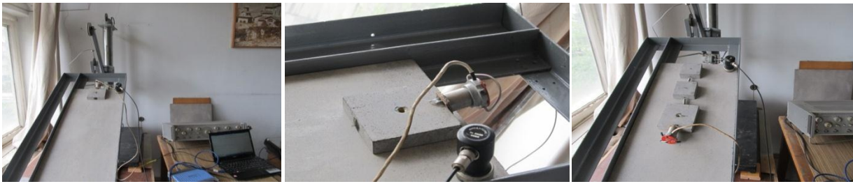
Fig. 4. Laboratory model for series of Burridge-Knopoff experiments under the influence of gravitational forces. Middle figure shows the seismic vibrator attached to the sliding plate.
