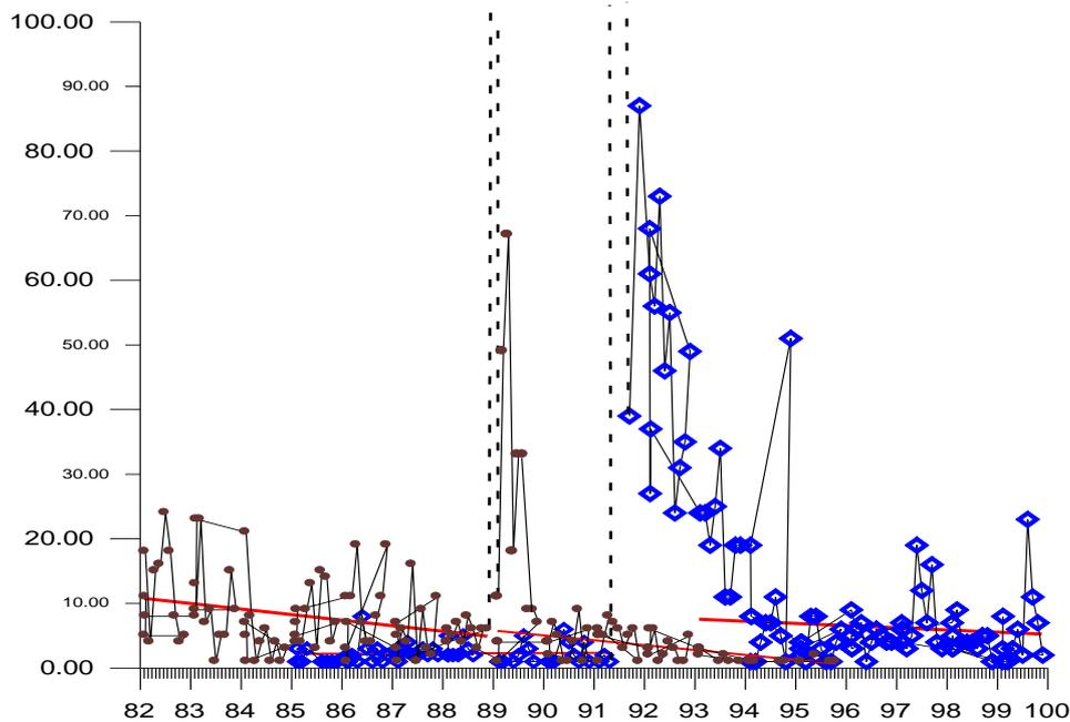
Fig. 9. The number of earthquakes for Racha earthquake of 1989 10 years earlier and after events (blue diamond). The number of earthquakes for Spitac earthquake of 1988 (brown dots). Redlines indicate the seismic level before and after earthquakes.
