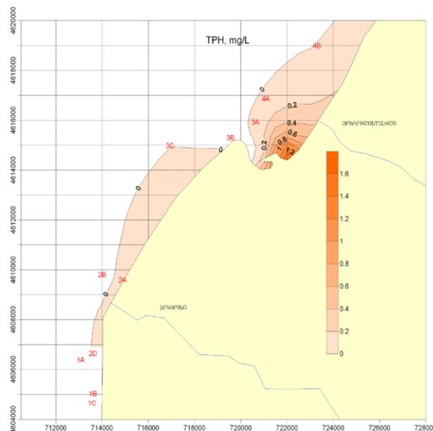
Fig. 3. Content of petroleum hydrocarbons in seawater at Gonio-Natanebi water area [14].
