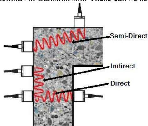
**Direct transmission:** Optimal configuration with maximum signal amplitude. The most accurate method for determining pulse velocity.
