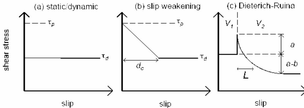
Fig.1. Friction laws for earthquake faults. (a) Static/dynamic friction. (b) linear slip weakening and (c) Dieterich-Ruina Rate and State law (Daub, 2009)
