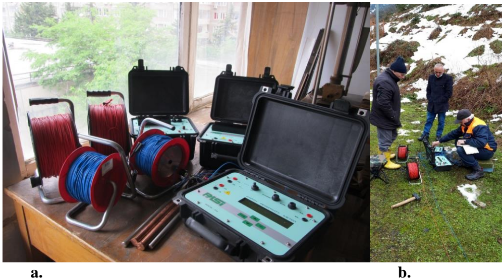
Fig.3. a) Earth Resistivity Meter PASI 16GL-N, b) measurement process.
