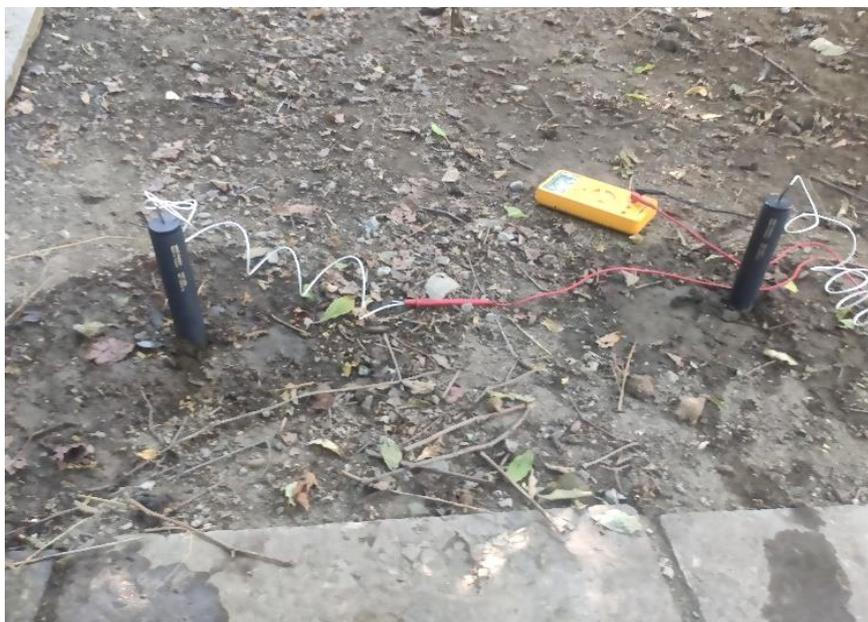
Fig. 6. Non-polarizable electrodes PMS 9000
