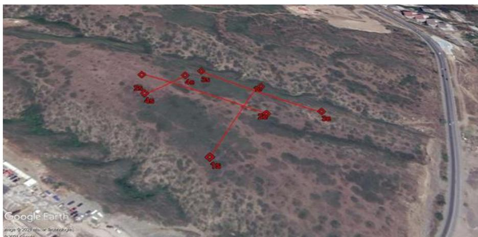
Fig.6. Layout scheme of seismic profiles. N s indicates the beginning of the profile, and N e - the end of the profile.
