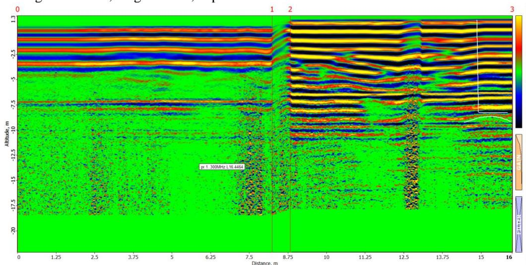
Fig. 2. Radargram Prof. 1 is presented, length - 16 m. It is made with a standard shielded radar antenna of 300MHz. The topographic effect is taken into account.
