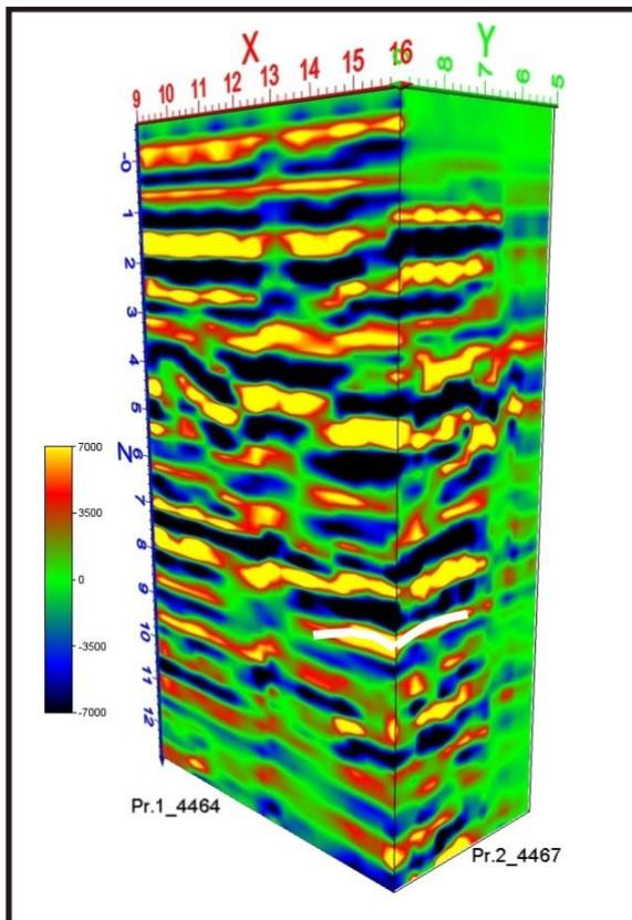
Fig. 6. An excerpt from the spatial representation of the intersection of profiles-1, 2 is provided. The 3D radio image is built using Voxler 4 software.
