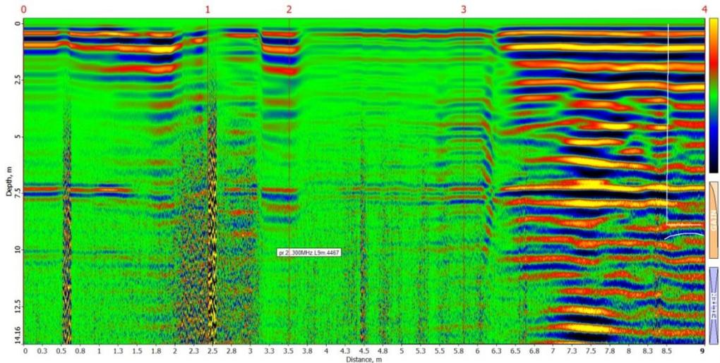
Fig. 3. Presents radargram Prof. 2, length -9m. It is made with a standard radar shielded antenna of 300MHz.
