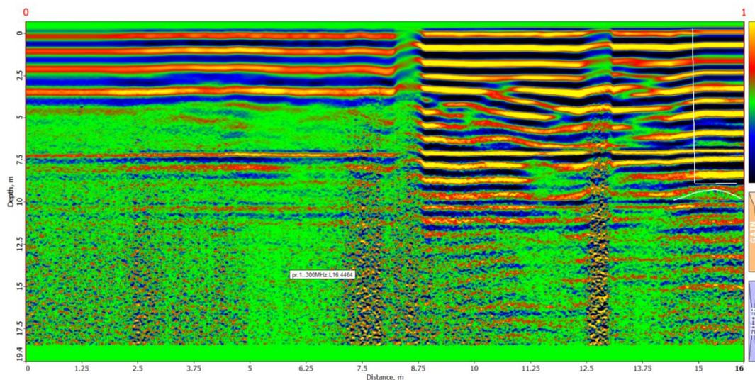
Fig. 1. Radargram Prof. 1, length - 16 m, is presented Zond-12e with standard shielded antenna 300MHz.
