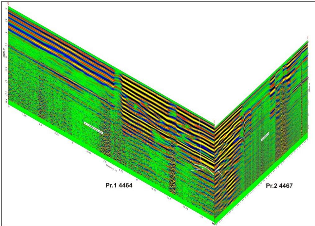
Fig. 5. Radargram Prof. 1 and Prof. 2 are presented, the target pile is located at the intersection, it is made with the radar staff screened antenna 300MHz.
