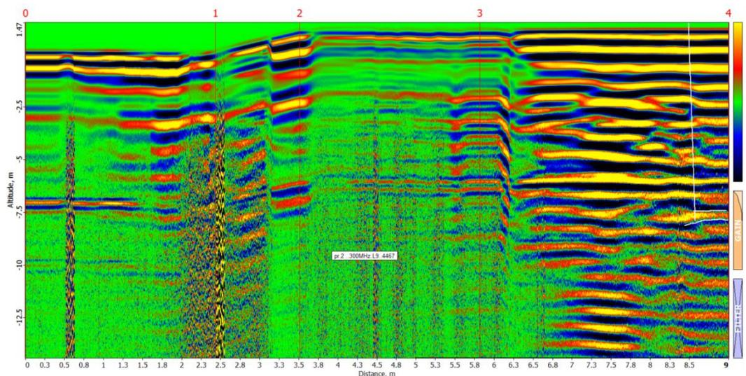
Fig. 4. Radargram Prof. 2, length -9m is presented. It is made with a standard radar shielded antenna of 300MHz. The topographical effect is taken into account.
