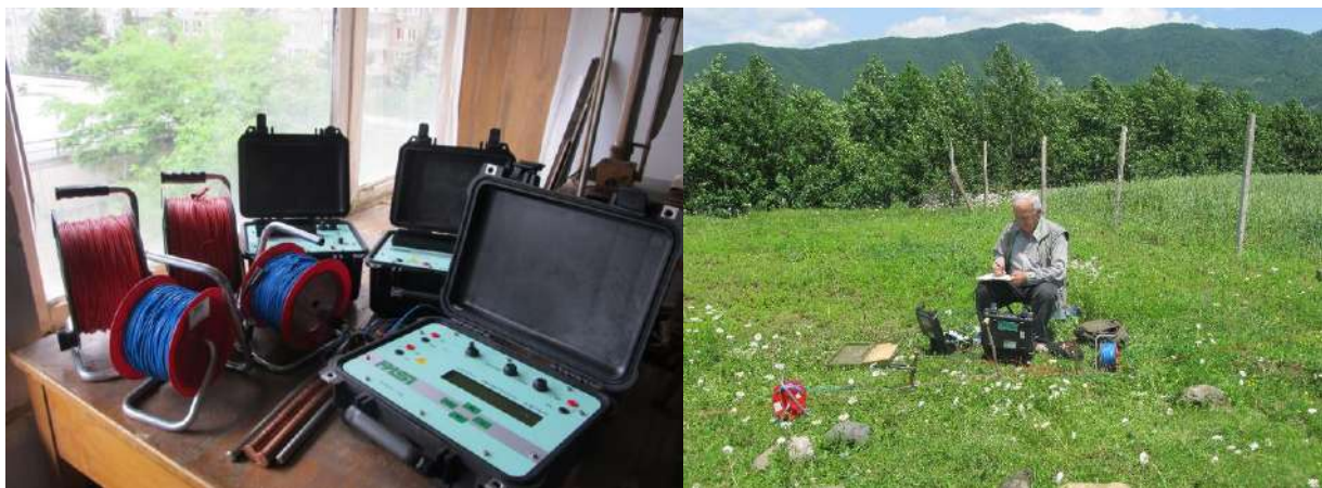
Fig.9. a) Earth Resistivity Meter PASI 16GL-N, b) measurement process
