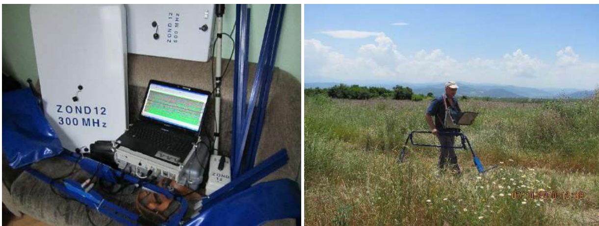
Fig.1. a) ground penetrating radar ZOND 12, b) measurement process
