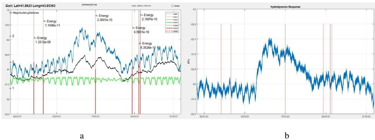
Fig.6. a - Water level, atmospheric pressure and tidal variations at the Gori borehole. Vertical line marks an earthquake. On abscise axis time is in hours. b- Hydrodynamic Response.
