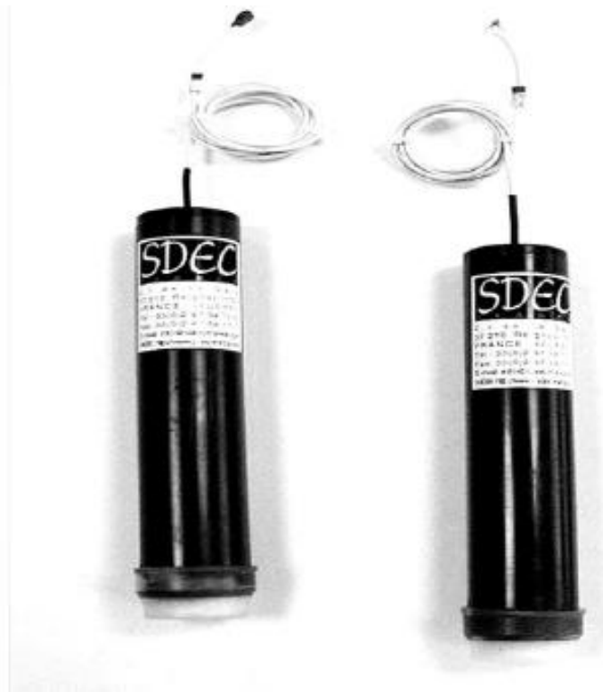
Fig. 2. Dry unpolarizable electrodes for self potentials measurement - PMS 9000
