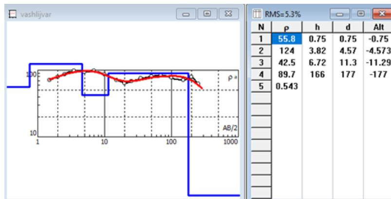
Fig. 4. Vertical electrical sounding curve obtained as a result of measurements on a landslide body.
