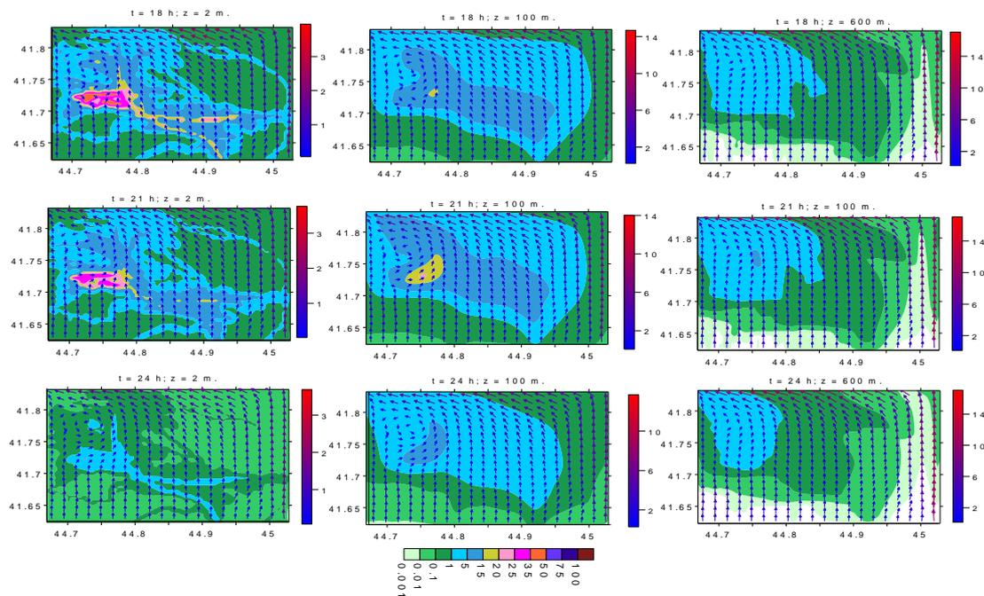
Fig. 6. Wind velocity (m/sec) and PM2.5 concentration ( $\text{mg/m}^3$ ) fields in summer, in the surface and boundary layers of the atmosphere, when  $t = 18, 21,$  and  $24$  h.
