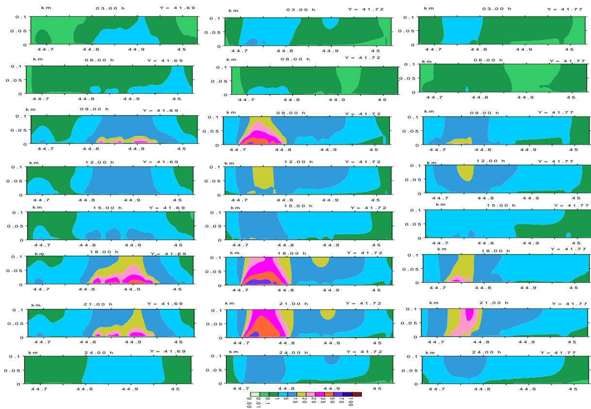
Fig. 7. PM2.5 concentration isolines in three vertical cross-sections made along the parallel in the lower 100 m thick atmospheric layer.
