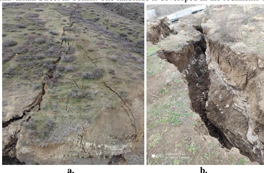
Fig. 1. a) Machavariani landslide photographed by drone, b) one of the ruptures of Machavariani landslide
