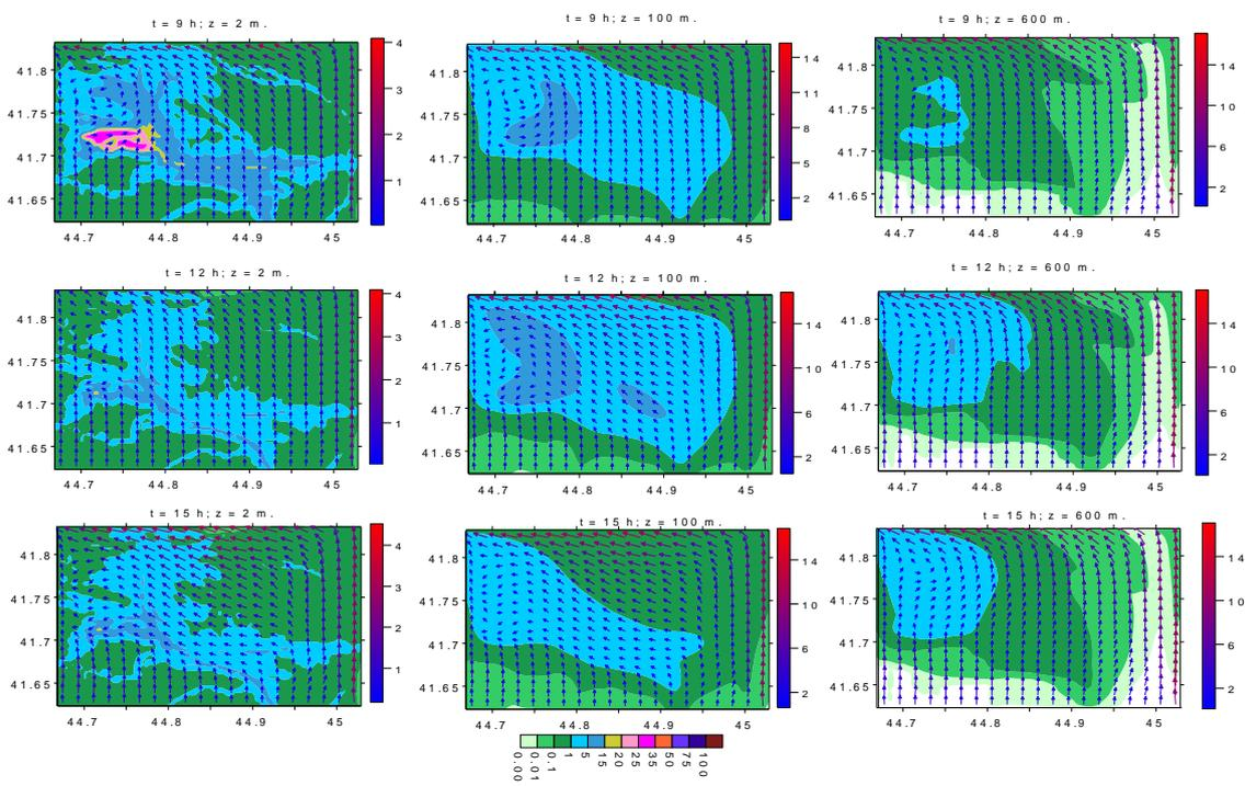
Fig. 5. Wind velocity (m/sec) and PM<sub>2.5</sub> concentration (mcg/m<sup>3</sup>) fields in summer, in the surface and boundary layers of the atmosphere, when t = 9, 12, and 15 h.
