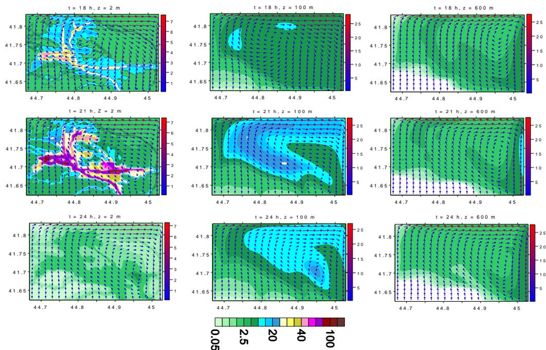
Fig. 8. Wind velocity (m/sec) and PM10 concentration (mcg/m<sup>3</sup>) fields in winter, in the surface and boundary layers of the atmosphere, when  $t = 18, 21,$  and  $24$  h
