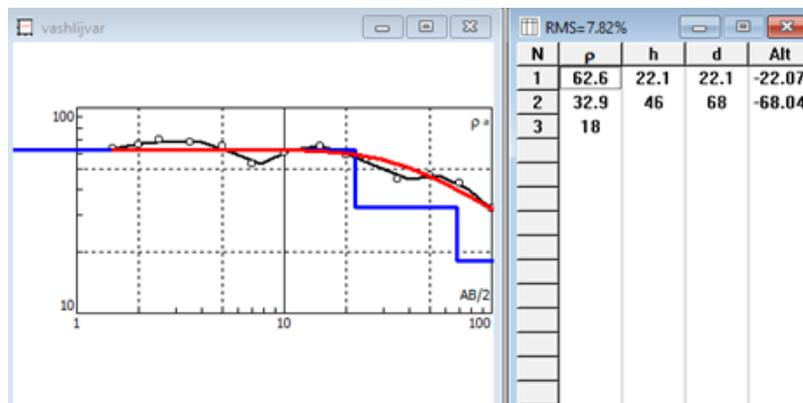
Fig. 3. Vertical electrical sounding curve obtained as a result of measurements near the landslide toe.
